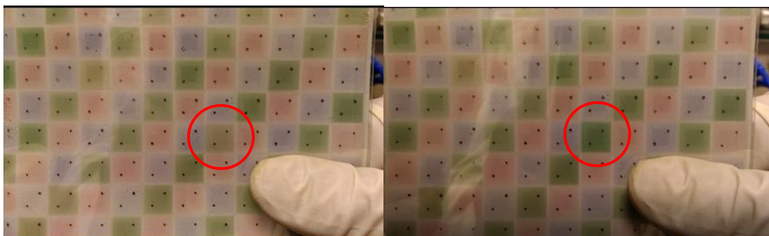
Figure 5. Individual pixel addressing is possible by creating through holes in one of the PET/ITO layer, while the other ITO electrode is grounded; color changes upon applied voltage from complete saturation to almost transparent state (with white backplane).
