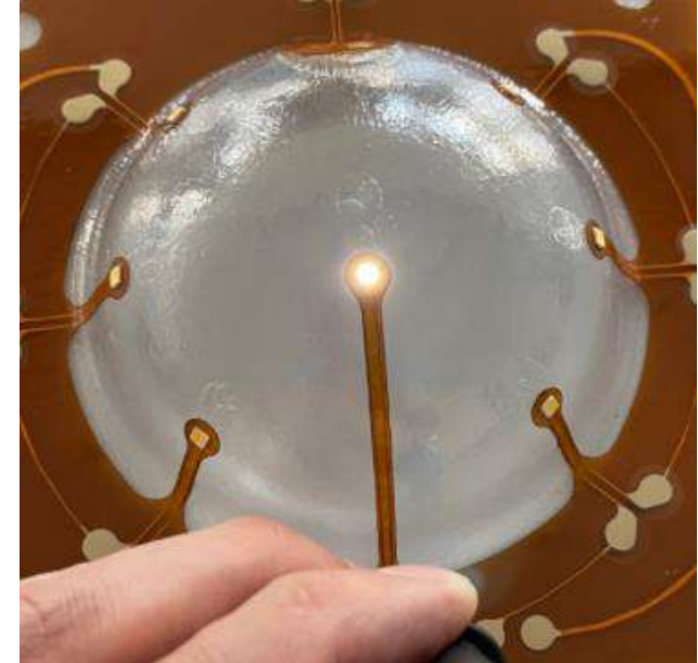
Functionality after thermoforming
