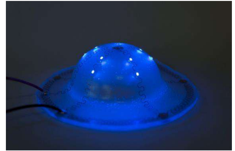
Stretchable circuit embedded in PC
