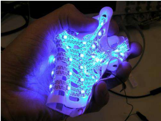
Stretchable circuit embedded in silicone
